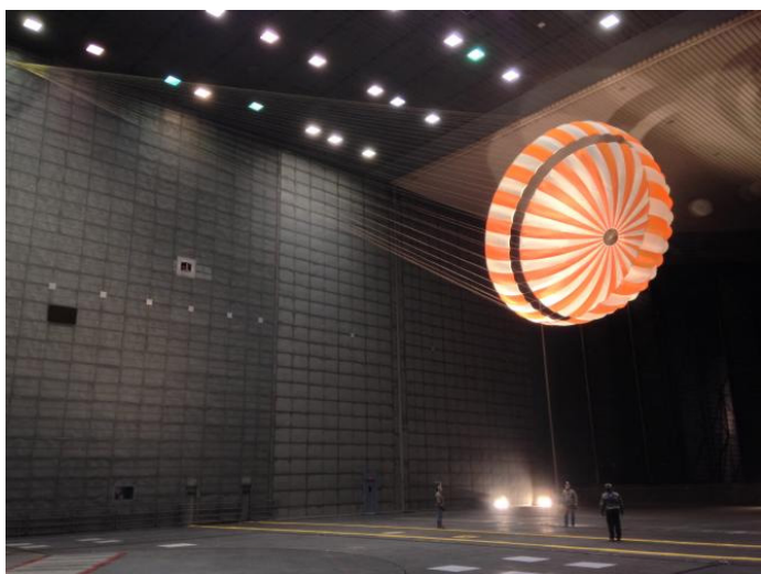
Parachute testing for InSight, conducted inside world's largest wind tunnel, at NASA Ames Research Center, Moffett Field, California.
