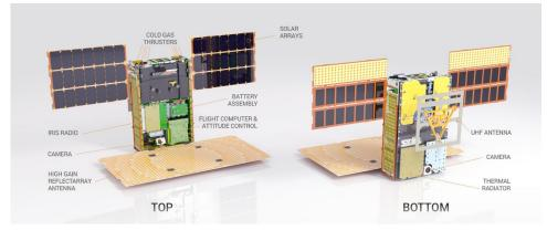
Illustration of one of the twin MarCO spacecraft with some key components labeled. Front cover is left out to show some internal components. Antennas and solar arrays are in deployed configuration.
