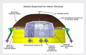
llustration of InSight's SEIS instrument with some key components labeled
