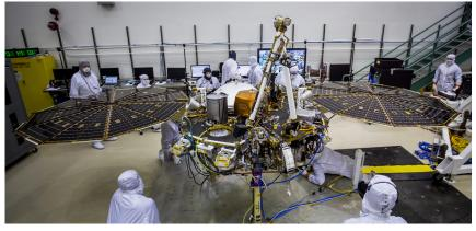
Engineers at Lockheed Martin Space, Denver, test the solar arrays on NASA's InSight lander several months before launch.
