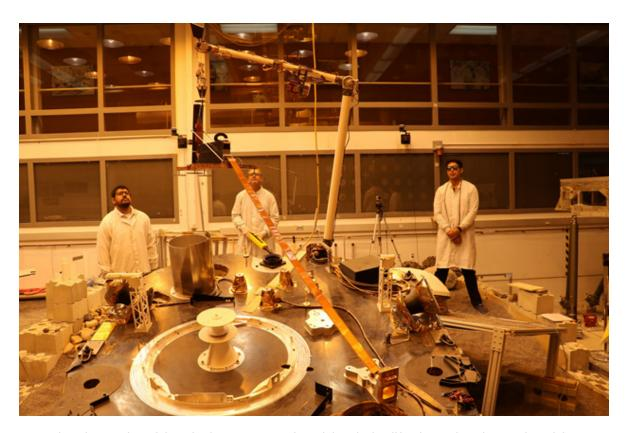
An engineering version of the robotic arm on NASA's InSight mission lifts the engineering version of the Heat Flow and Physical Properties Probe (HP³) at NASA's Jet Propulsion Laboratory.
