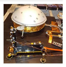
HP<sup>3</sup> (foreground) and domed Wind and Thermal Shield (covering SEIS) in preparation for thermal vacuum testing. Credit: NASA/ JPL-Caltech/Lockheed Martin Space
