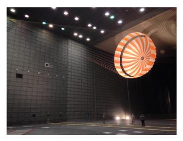
Parachute testing for InSight, conducted inside world's largest wind tunnel, at NASA Ames Research Center, Moffett Field, California.
