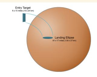
Navigators' target at the top of Mars' atmosphere is smaller than the ellipse covering the area in which the spacecraft has a 99 percent chance of touching down after passing through that target. Dispersion factors include aerodynamic uncertainties and atmospheric variability. This concept illustration is not to scale.
