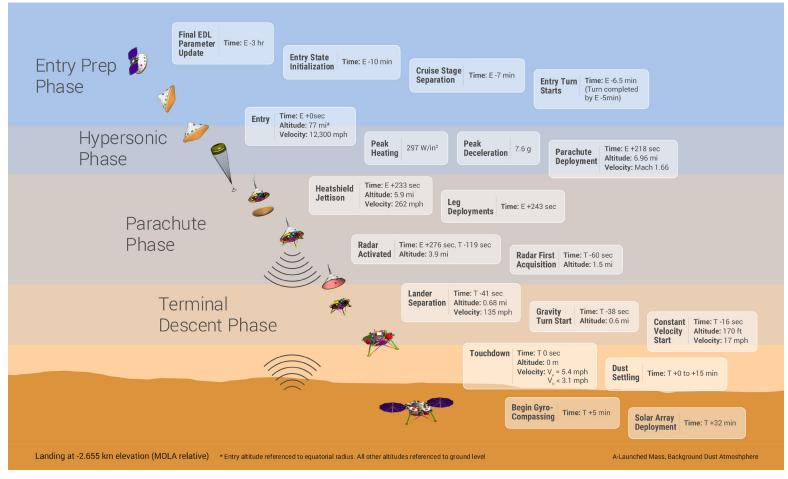
Profile of InSight entry, descent and landing events on Nov. 26, 2018, for one typical case. Exact timing will be affected by atmospheric conditions on landing day.
