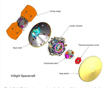
The InSight flight system comprises the lander, with its component deck and thermal enclosure cover, encapsulated in the aeroshell formed by the back shell and heat shield, and topped by the cruise stage. Credit: NASA/JPL-Caltech/Lockheed Martin Space
