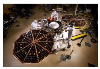
The solar arrays on NASA's InSight lander are deployed in this test in a clean room at Lockheed Martin Space, Denver, in April 2015. Each of the two arrays is 7.05 feet (2.15 meters) in diameter.
