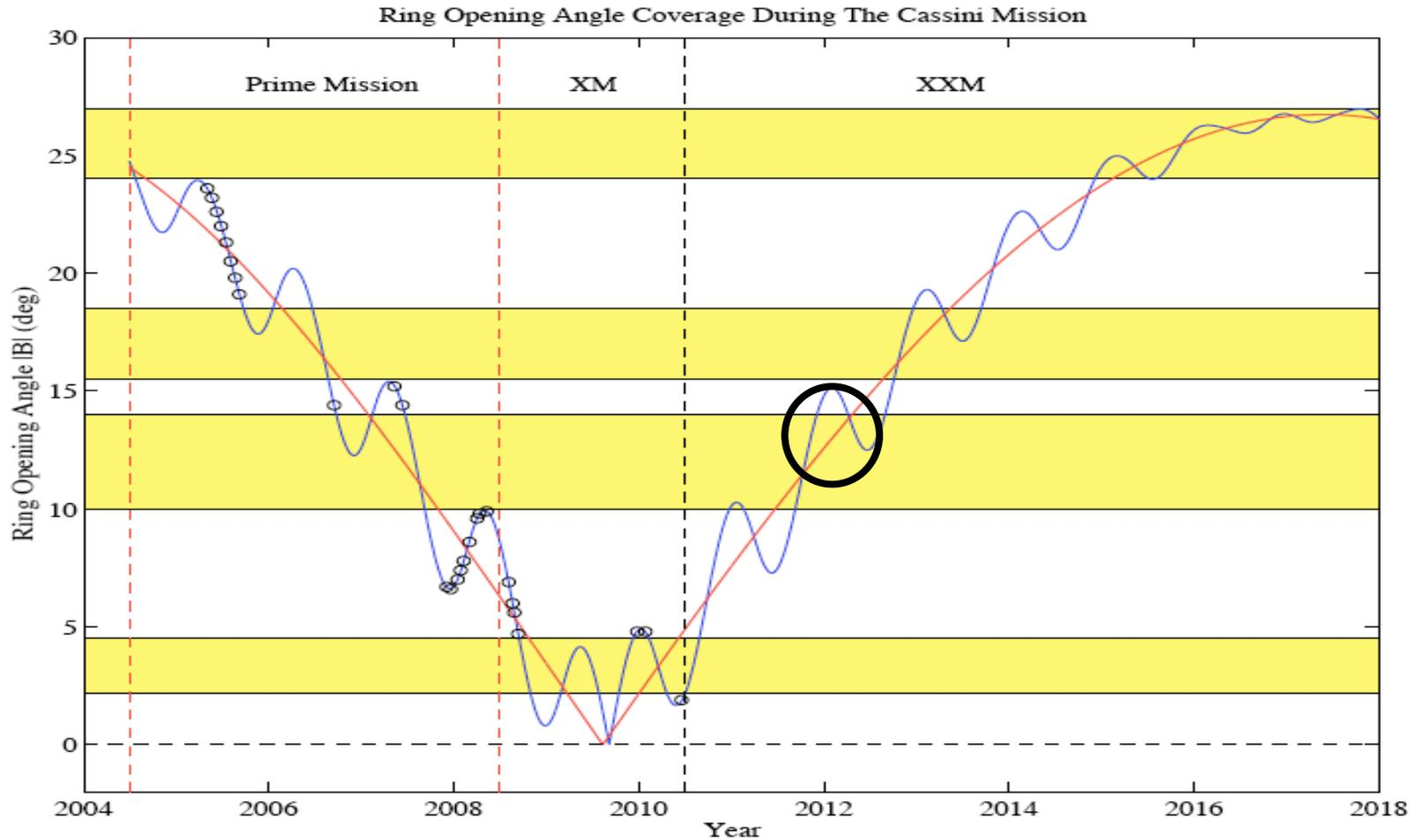
Opening angle affects insolation, ring temperature, RSS transmission, spoke occurrence frequency, diffuse ring structure
