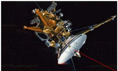
The spacecraft turns to Earth for a typical 9 hour tracking pass, to downlink telemetry data and receive commands.
