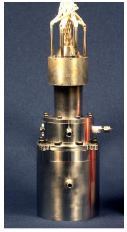
Figure 3-6. Laboratory Prototype of an Advanced 80 We SunPower Stirling Engine and Linear Alternator (Wood, 2005).
