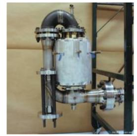
Figure 3-7. 1-kWe Engine and Resonator Developed by NGST and LANL (Petach, 2004b).
