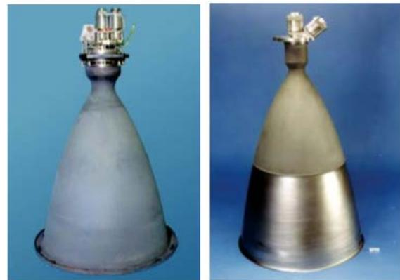
**Figure B-24:** R-40B 4,000N and R-4D-15 450N (HIPAT) rocket engines (not to scale).
