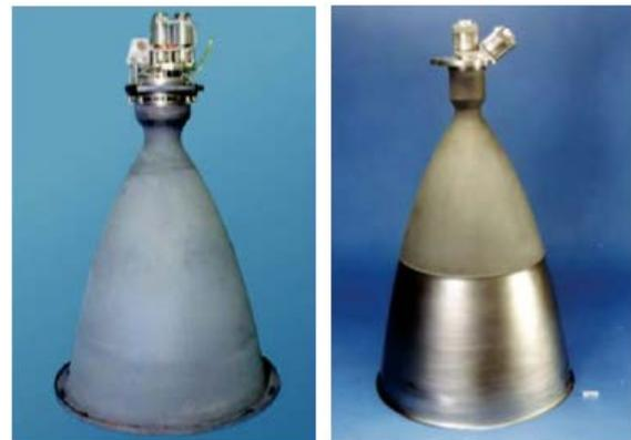
**Figure B-46:** R-40B 4,000N and R-4D-15 450N (HiPAT) rocket engines (not to scale).
