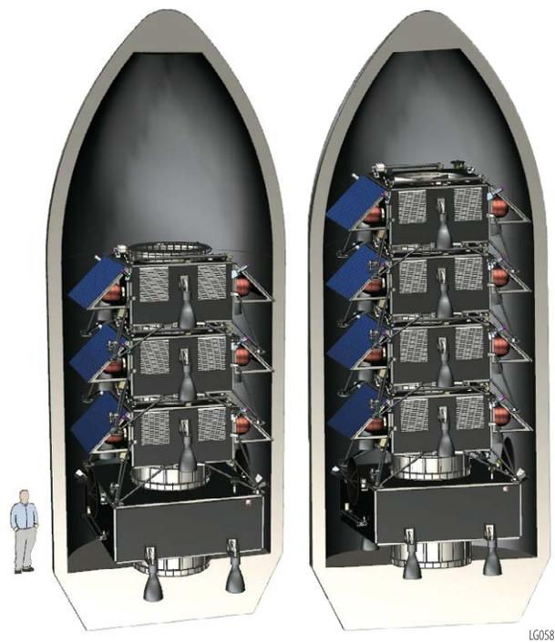
Figure B-22: LGN Three Lander Launch Configuration (left), LGN Four Lander Launch Configuration (right).
