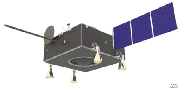
**Figure B-41:** LGN Orbiter communication relay deployed configuration.
