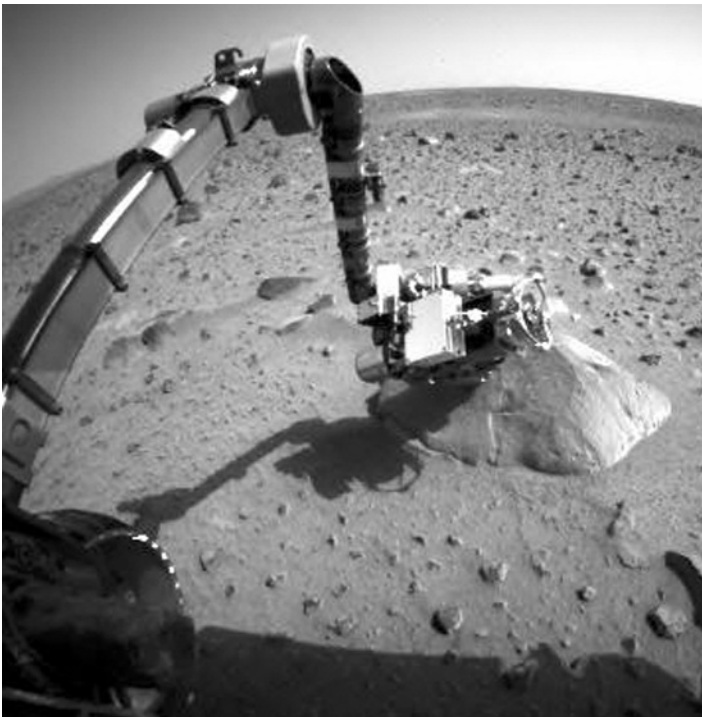
Spirit's robotic arm reaching to a rock informally named "Adirondack" for examining the rock with tools on the arm.
