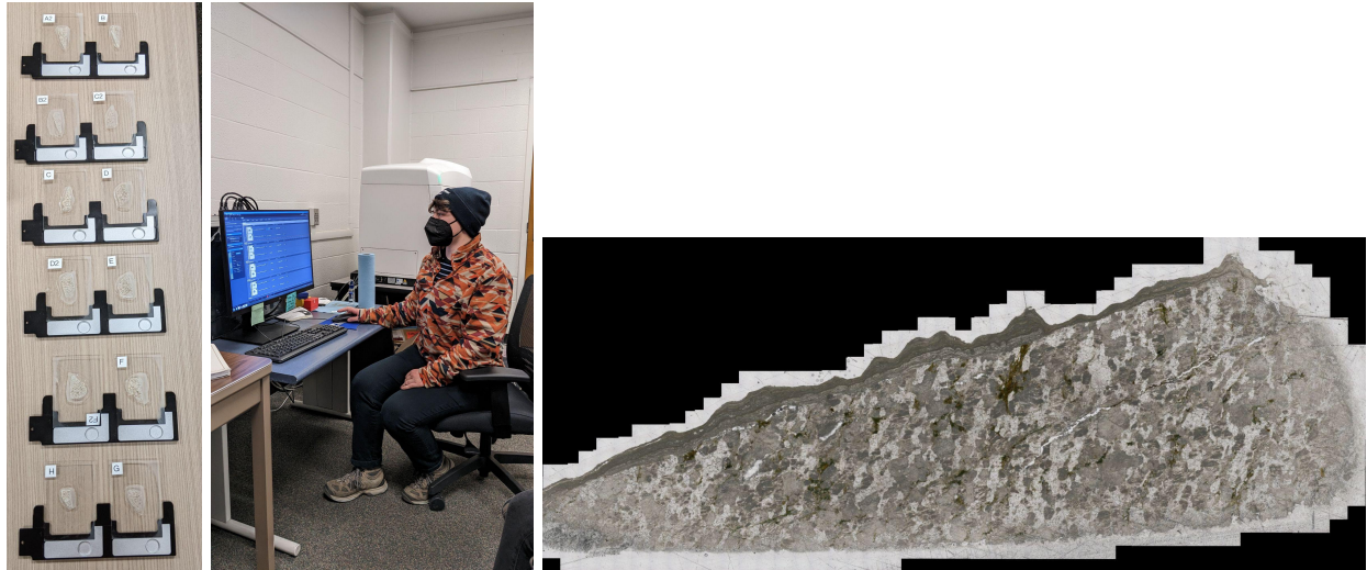
Figure 1: Thin sections being prepared for imaging using the Zeiss AxioScan.Z1 fully-automated slide scanner (left). PhD candidate Schuyler Borges using the slide scanner software to prepare samples for imaging (middle). Image of a thin section from the Zeiss AxioScan.Z1 fully-automated slide scanner (right).
