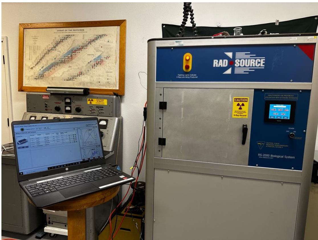
Figure 1. X-ray irradiation system equipped with oxygen sensors positioned inside the irradiation chamber (right) for real-time monitoring of photosynthetic oxygen production on the computer (left) during X-ray exposure.
