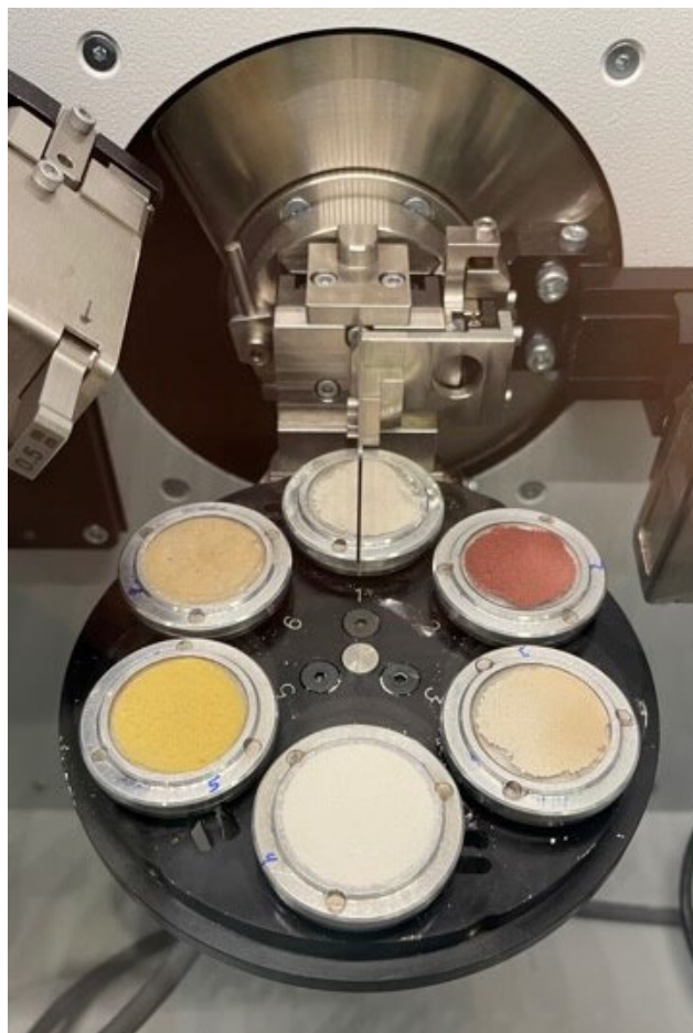
Figure 1. Western Australia lake samples were dried (if needed), powdered, and then processed by XRD, shown in this image.
