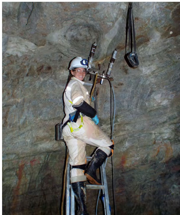
Fig. 1 - Rachel Harris successfully installs cell incubation and lipid cartridges to the front arms of the prawn at BE326-BH2 one mile beneath the surface. A methanometer is hanging next to her. Photo by: T.C. Onstott
