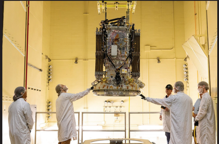
Engineers from Katalyst stabilize their LINK robotic servicing spacecraft as it moves into a vibration chamber at NASA's Goddard Space Flight Center in Greenbelt, Md., on April 15, 2026. The vibration chamber simulated the intense shaking LINK will experience during launch. Credit: NASA/Scott Wiessinger
