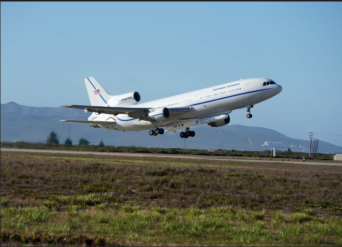
Northrop Grumman's Stargazer, a modified L-1011 aircraft, takes off from Vandenberg Air Force Base in California. The company's Pegasus XL rocket, carried beneath the aircraft as shown here, will launch Katalyst's LINK spacecraft. Credit: Northrop Grumman
