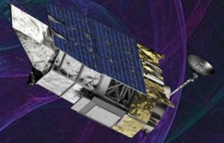
**Hubble-Like Resolution** ~0.1" **Near-Infrared Imaging and Spectroscopy** 0.48–2.3  $\mu\text{m}$  **Expansive Field of View** 0.281 deg<sup>2</sup> **All Data Nonproprietary** ~4 Pb/yr
