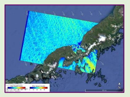
The radar cross section, or brightness, of a synthetic aperture radar (SAR) image can be related to wind speed. Above is an image of wind speed over the Alaskan Peninsula derived from Sentinel-1B SAR data. The various wind speeds are represented as different colors. NISAR will be able to provide similar wind speed measurements in coastal areas. NOAA regularly generates wind speed products using available SAR data, and NISAR will augment the available information, particularly along U.S. coasts.
