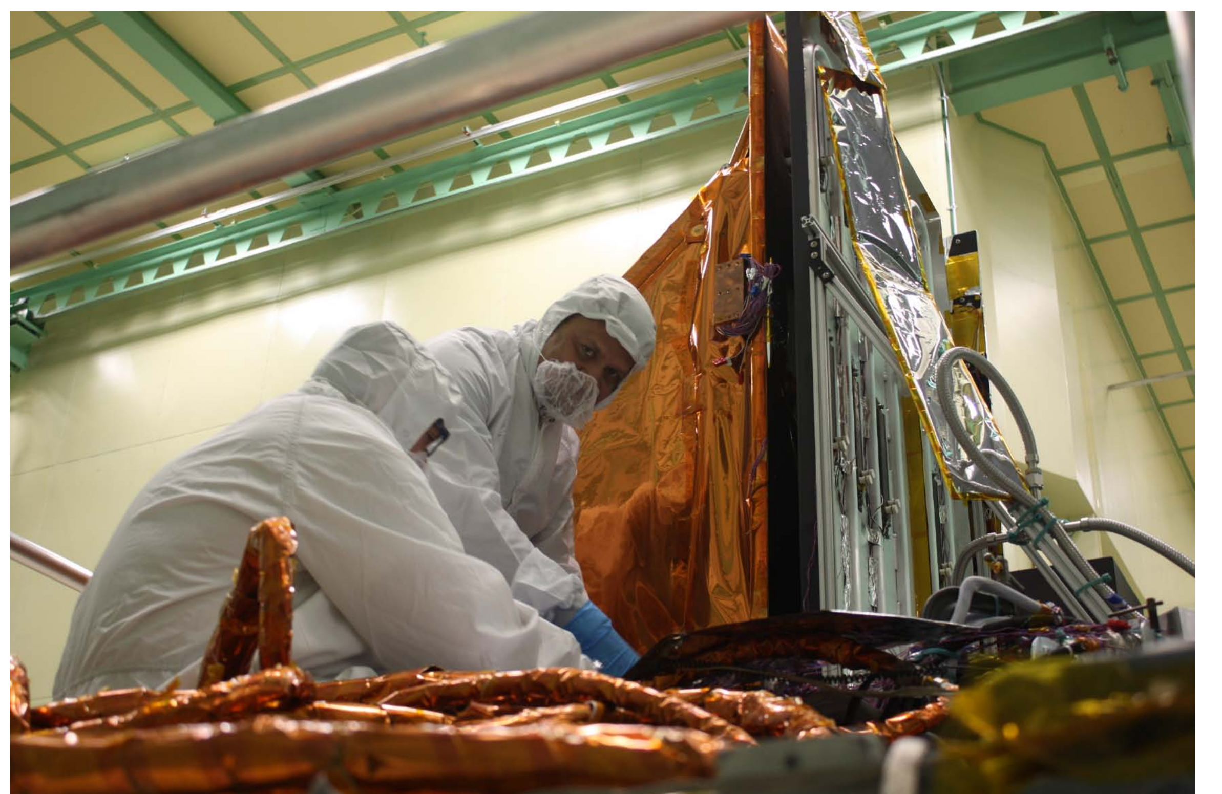
Below, engineers cover the Thermal Infrared Sensor with insulation blankets in the final stages of assembling it.
