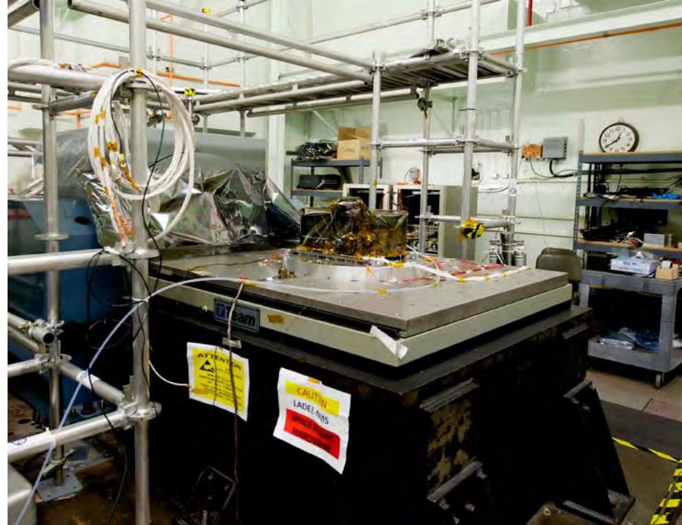
The "shaker table" at NASA Goddard Space Flight Center
