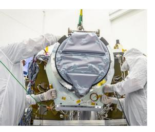
Tim Lippy of the Johns Hopkins Applied Physics Laboratory in Laurel, Maryland, and Marc Miller of the Laboratory for Atmospheric and Space Physics (LASP) install the IDEX instrument to the Interstellar Mapping and Acceleration Probe. Credit: NASA/Johns Hopkins APL/Princeton/Ed Whitman
