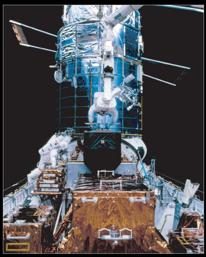
Giving Guidance: Replacing the Fine Guidance Sensors
