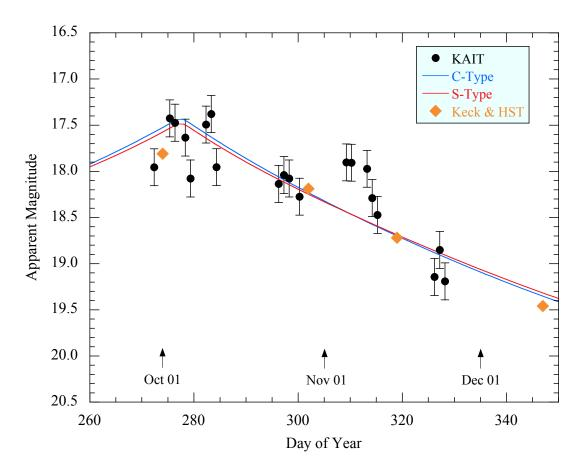
Fig. 2.— R-band photometry from KAIT (black circles) and from Keck and HST (orange diamonds) within a 6" radius circular aperture as a function of Day of Year in 2013. Lines show the brightness variation expected of an asteroid following the inverse square law of distance and with phase functions appropriate for C-type (blue) and S-type (red) surfaces.
