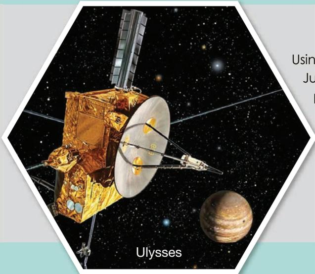
Using RTGs, Ulysses completed three rendezvous with Jupiter between 1992 and 2008, utilizing the giant planet's gravity to accomplish three passages over the Sun's north and south poles.
