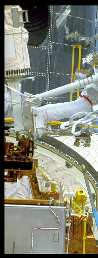
During Hubble's first servicing mission, astronaut Jeffery Hoffman removed the Wide Field and Planetary Camera 1, before replacing it with its successor. The camera, wedge-shaped and similar in size to a mini-grand piano, weighed 610 pounds on Earth, but nothing in space. However, it has the same mass and momentum as on Earth, so Hoffman had to be extra careful moving it!
