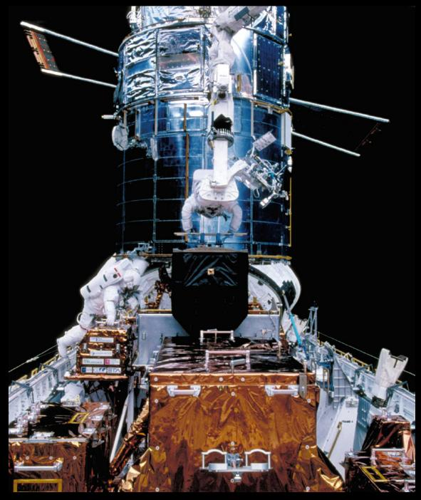
Astronauts Joseph Tanner and Gregory Harbaugh replaced Hubble's Fine Guidance Sensors during Servicing Mission 2. The Fine Guidance Sensors locate and lock onto a guide star while science instruments make observations of an astronomical object or phenomenon.
