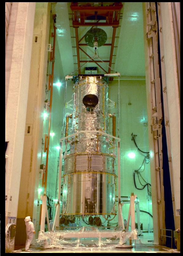
The Hubble Space Telescope lifted into an upright position in Lockheed Martin's acoustic vibration chamber for pre-launch testing.
