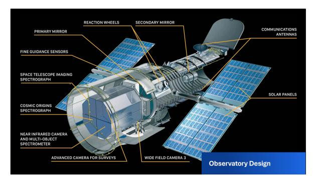
The observatory is powered by two solar arrays that convert sunlight into electrical energy that is stored in six large batteries. The batteries allow the observatory to operate during the shadowed portions of Hubble's orbit when Earth blocks the satellite's view of the Sun.
