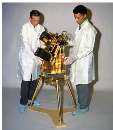
Dr. George Carruthers, right, and William Conway, a project manager at the Naval Research Institute, examine the gold-plated ultraviolet camera/spectrograph, the first Moon-based observatory that Carruthers developed for the Apollo 16 mission. Apollo 16 astronauts placed the observatory on the moon in April 1972.
