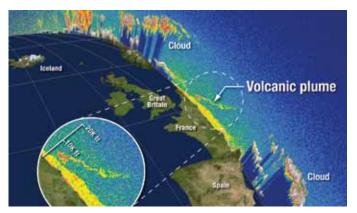
Lidar sends infrared light pulses and measures the reflection and scattering to image the distribution of aerosols and gases in the atmosphere.
