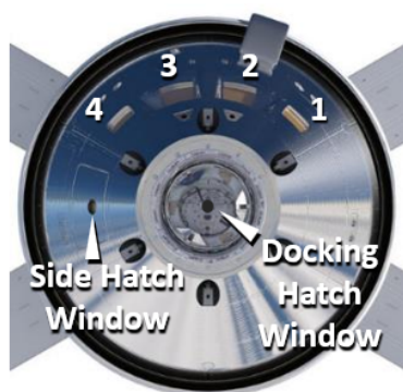
Figure 2. Orion vehicle observing windows: forward Windows 1, 2, 3, and 4, Side Hatch, and Docking Hatch.
