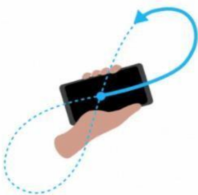
Figure 4. Calibration of smart device magnetometers using the ‘figure 8’ method.
