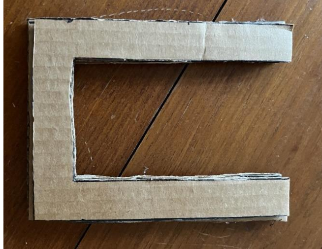
Figure 23. Example of a completed 3-layer U-shaped flange.
