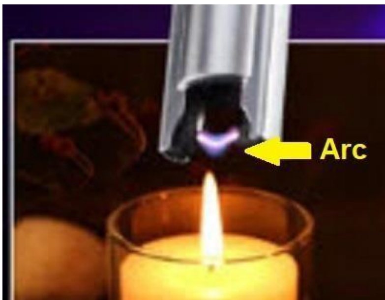
Figure 37. Electric arc lighter with plasma. The plasma is contained in the blue arc between the electrodes.
