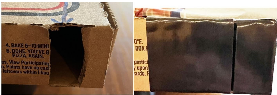
Figure 17. Installing the Slit. Left) Cut a 25 mm wide hole. Right) Cover the hole with tape to form the Slit.
