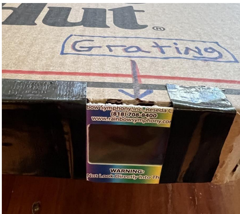
Figure 16. Grating trimmed and installed on the wall of the box.
