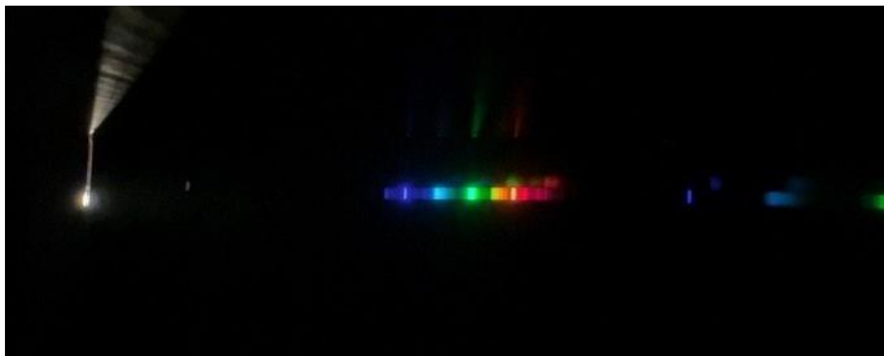
Figure 26. Example of CFL spectrum with TimeStampCamera app (Apple: free ). Note the wide-angle view lets you use the image of the lamp through the slit on the far Left, and the spectrum in the center
