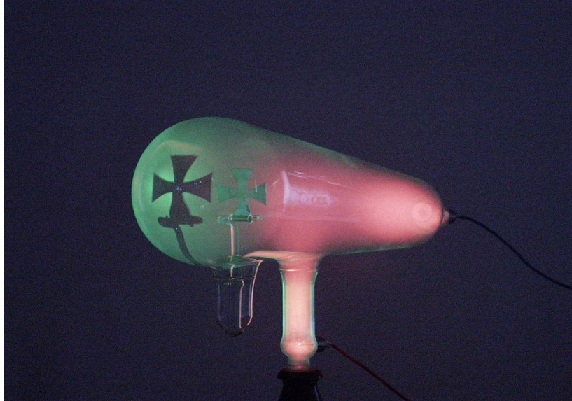
Figure 1. Crookes tube showing glow. (Credit: Wikipedia/Zátonyi Sándor)
