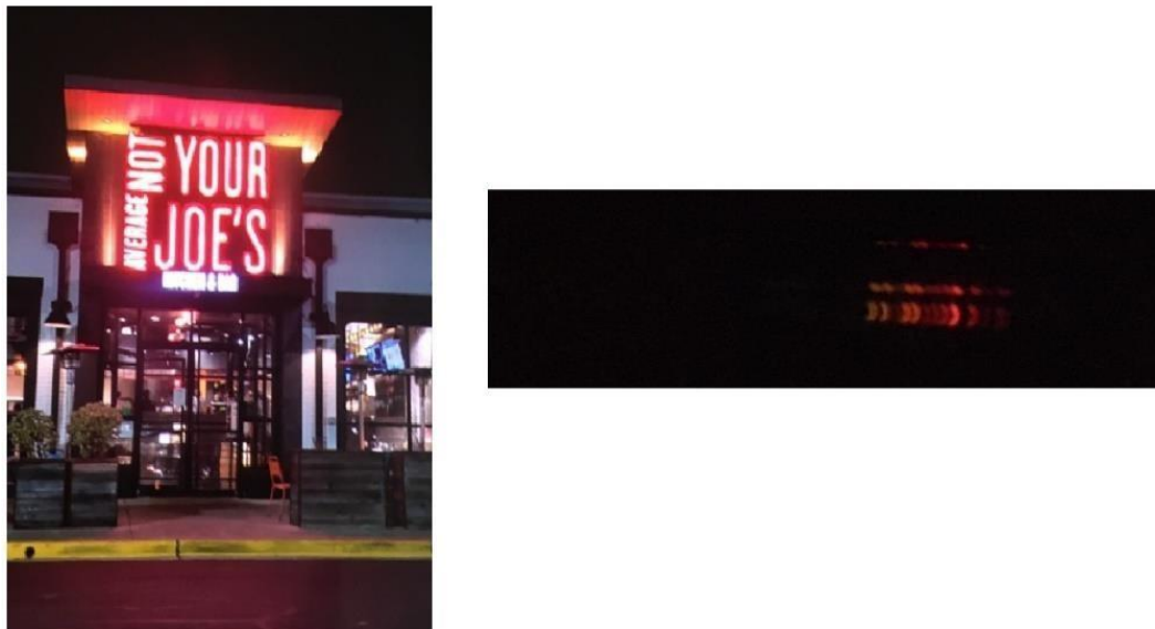
Figure 32. Neon signs produce only limited spectral lines as the neon plasma is heated. Each of the spectral lines takes the shape of the gas emitting the light, which is why the lines in the figure are wavy and not straight.
