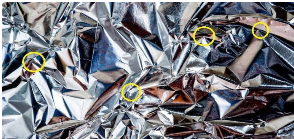
Figure 40. Crumpled aluminum showing spark and details. The yellow circles show places where adjacent corners are closer than one millimeter. This is where sparks will form.
