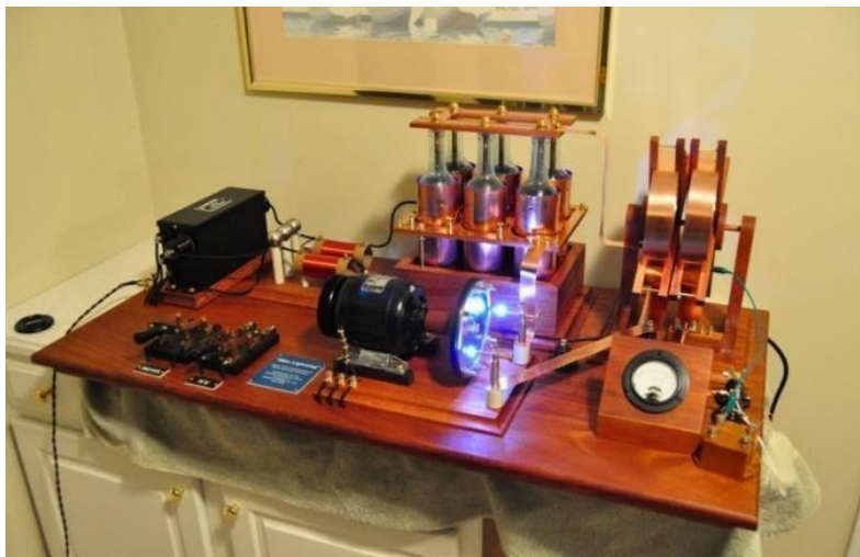
Figure 7. A spark gap transmitter. The blue glow is the plasma arc produced by the powerful battery circuit. These transmitters have been illegal to operate since 1934 because they interfere with other frequencies used by modern radio receivers. (Credit: Ian Poole; DxZone.com)
