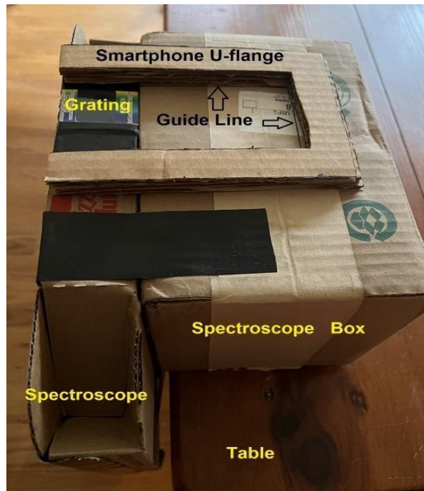
Figure 24. U-flange installed in the grating area using guidelines.
