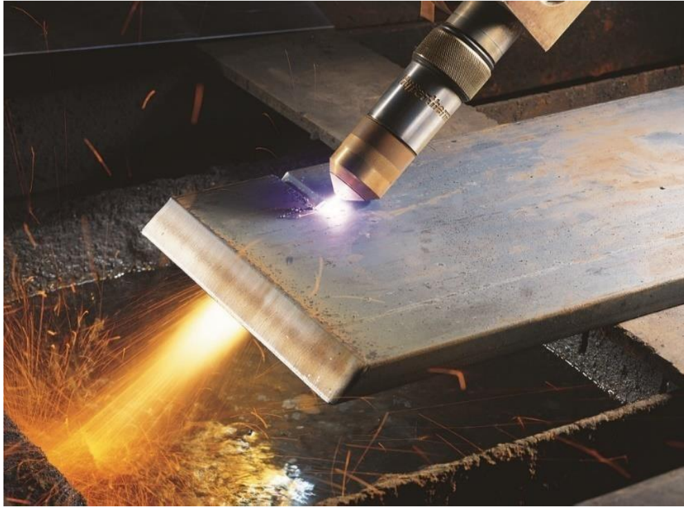
Figure 38. Example of an industrial plasma torch cutting steel. The plasma has a temperature of 15,000°C and cuts through metal like a hot knife cuts through butter .
