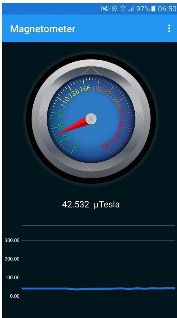
Figure 11. A smart device display showing the screen for the Magnetometer Metal Detector (Sylvain Saurel, Android). It indicates a magnetic field strength of 42.532 \mu\text{T} , but students can round-up the value to 42.5 \mu\text{T} because the additional decimal points are not needed for experiments in this guide.
