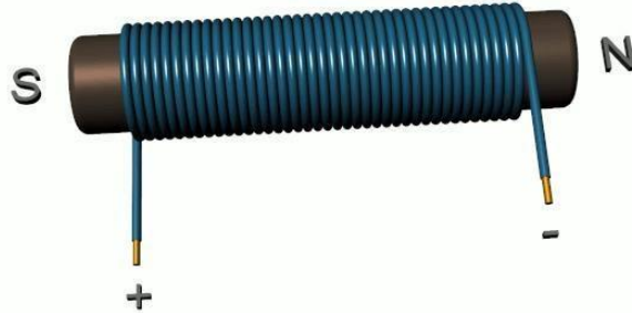
Figure 25. The number of loops of wire determine the strength of an electromagnet. The direction of current flow (positive to negative) also determines the polarity. (Credit: Wikipedia)
