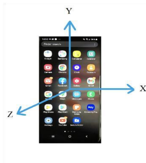
Figure 5. Body Frame coordinates for smart devices showing the axis labels and the direction of positive change. The origin of the coordinate system is at the middle of the phone casing.
