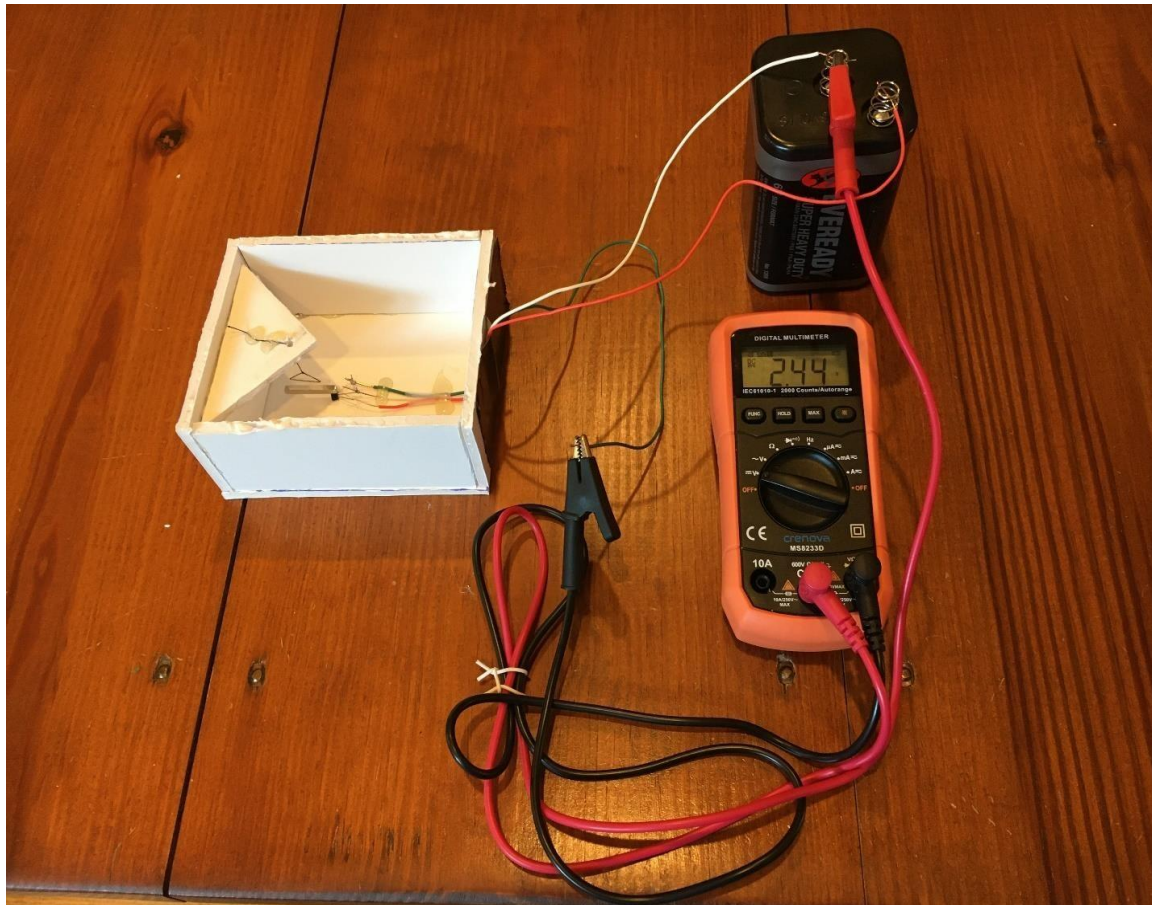
Figure 7. Measuring set up for the Hall sensor magnetometer. White wire is the ground Battery – and the red meter lead. Red wire is V+, and Battery+. The Green wire is clipped to the black meter lead.
