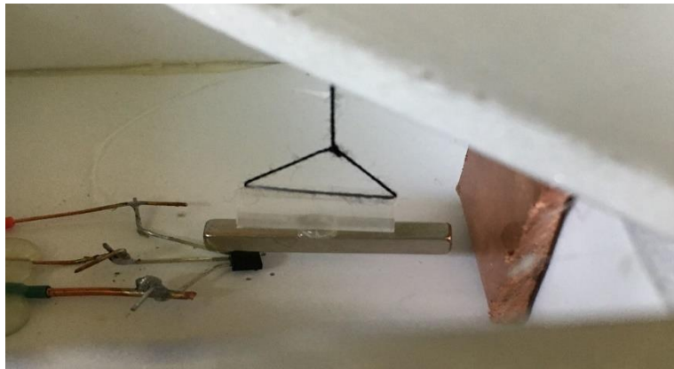
Figure 17. Magnetic damper installed near bottom-mounted magnet sensor. Note that when the magnet is in the Null position pointing due-North (magnetic), the magnet axis is perpendicular to the copper plate damper.
