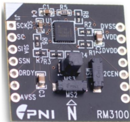
Figure 8. The RM3100 development board with the three magnetometers; one for each axis.
