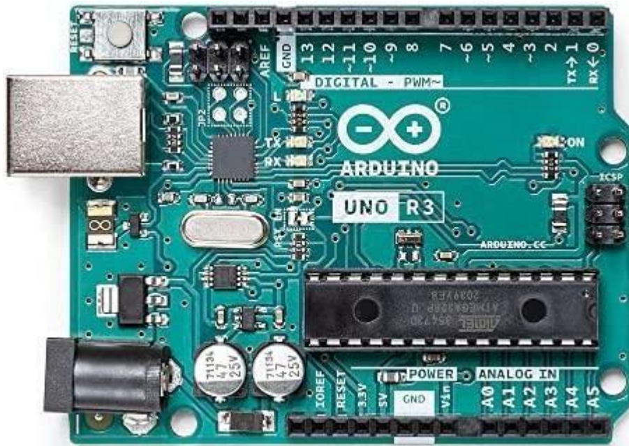
Figure 2. The Arduino 'Uno' microcontroller board.
