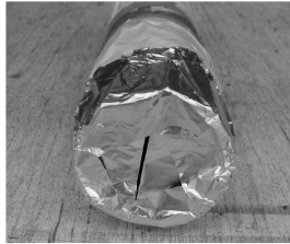
The slit end of a spectroscope. This end points at your light source.
