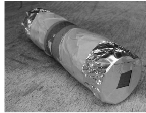
The diffraction grating end of a spectroscope. This end goes up to your eye
