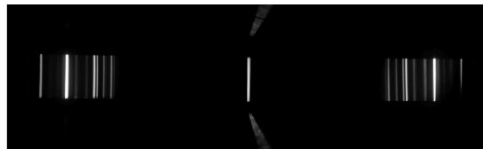
These nice orderly lines represent a fully aligned spectroscope. If this is what you are seeing through yours, you can tape the slit end in place.
