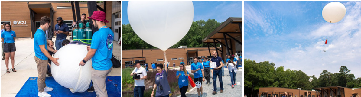
Photo 3. Students and scientists from NASA's Goddard Space Flight Center launch an ozonesonde. Shortly after the launch, the team studied the data the balloon collected, detecting higher levels of pollution in the atmosphere as smoke from wildfires in Canada drifted over the East Coast. Image credit: VCU
