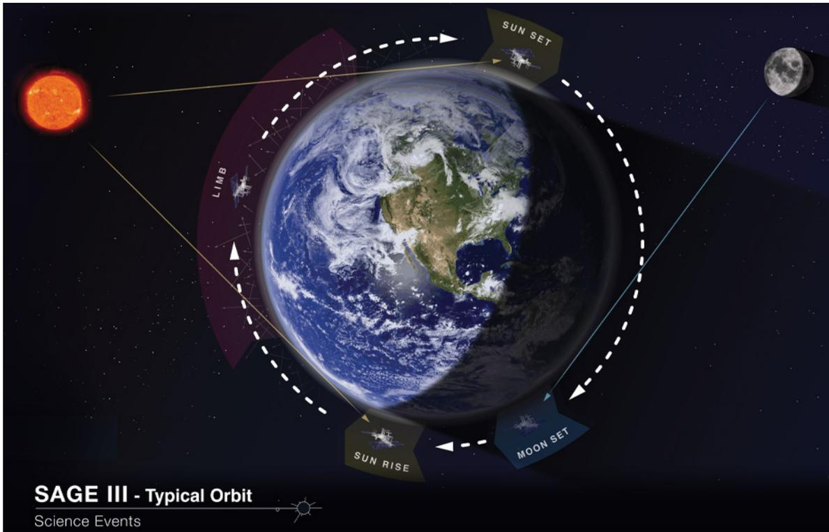
**Figure 2.** The SAGE III instrument takes measurements around the globe using a technique called occultation. Every time the Sun or Moon rises and sets (which, on ISS, occurs 15–16 times each day), SAGE uses the light that passes through the atmosphere to measure gases and particles in that region of the atmosphere. **Figure credit:** NASA
