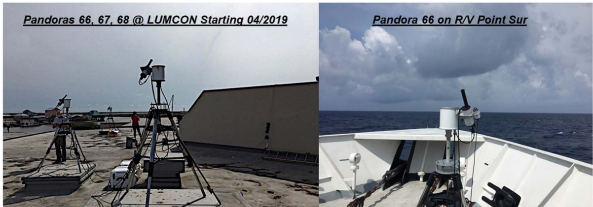
Figure 4. [Left] The three Pandora spectrometers during the calibration and intercomparison period on the roof of the Louisiana Universities Marine Consortium (LUMCON) building from April 10–May 8, 2019. [Right] On May 9 Pandora 66 was moved to the bow of the R/V Point Sur to collect measurements from the ship during the SCOAPE cruise. Photo credits: Ryan Stauffer
