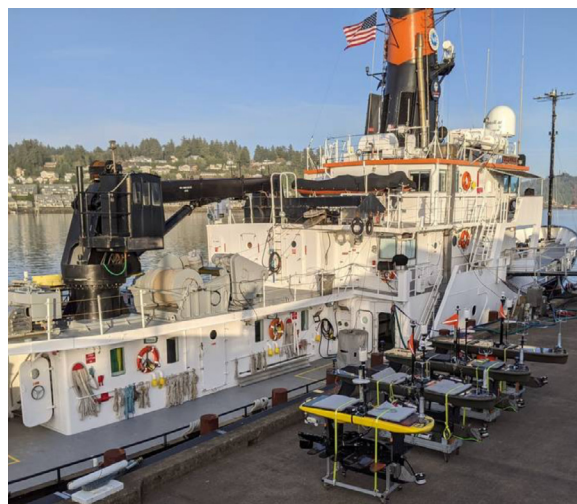
Photo 1. Several autonomous marine robots, including these Wave Gliders from Scripps Institution of Oceanography and the Woods Hole Oceanographic Institution, will deploy from R/V Oceanus . Credit: Laurent Grare/Scripps Institution of Oceanography
