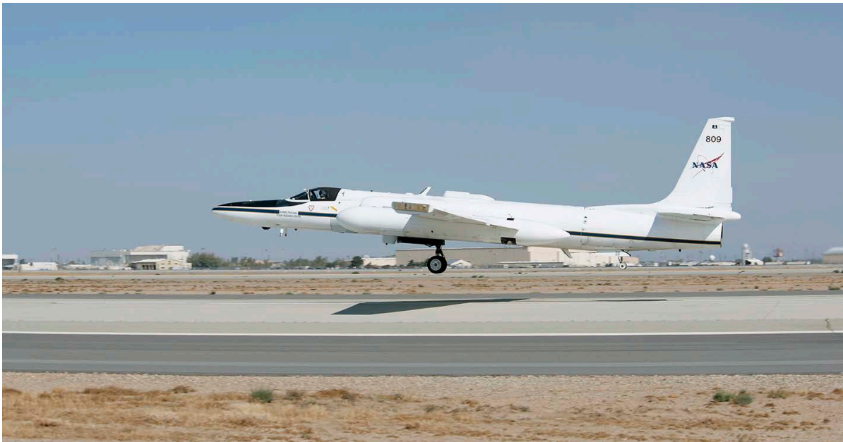
Figure 3. NASA's high-altitude ER-2 aircraft will make flights during ORACLES at 65,000 feet (~20 km) with instruments that make measurements similar to those acquired from satellites. Image credit: NASA
