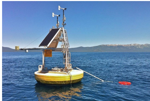
Figure 1. A combination of satellite data and ground measurements, such as from instrumented buoys like this one in Lake Tahoe on the California/Nevada border, were used to provide a comprehensive view of changing lake temperatures worldwide. The buoy measures the water temperature from above and below. Image credit: Limnotech
