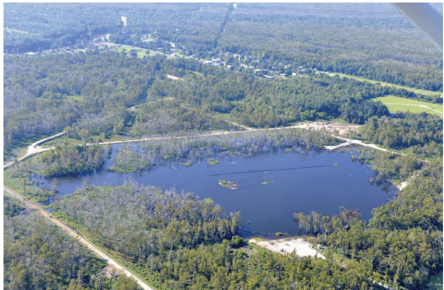
This is an aerial photo of a 25-acre (10-hectare) sinkhole that formed unexpectedly near Bayou Corne, LA, in August 2012. New analyses of NASA synthetic aperture airborne radar data collected in 2012 reveal the radar detected indications of the sinkhole before it collapsed and forced evacuations. Such data may someday help foresee sinkholes. Image credit: On Wings of Care , New Orleans, LA
