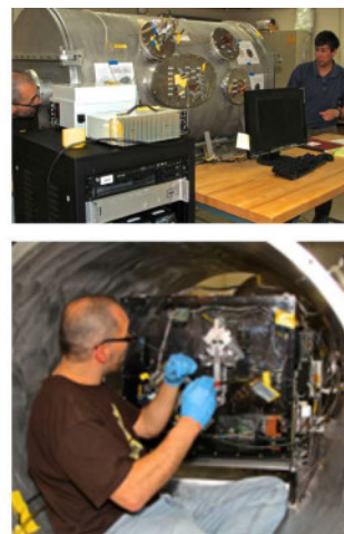
Figure 1. Shown here is the UW Absolute Radiance Interferometer (ARI) Prototype with On-orbit Verification and Test System (OVTS) technologies in thermal vacuum testing. The prototype features an On-orbit Absolute Radiance Standard (OARS) cavity blackbody, On-orbit Cavity Emissivity Module (OCEM), On-orbit Spectral Response Module (OSRM), and calibrated blackbodies: the ambient blackbody (ABB) and the hot blackbody (HBB). Image credit: UW
