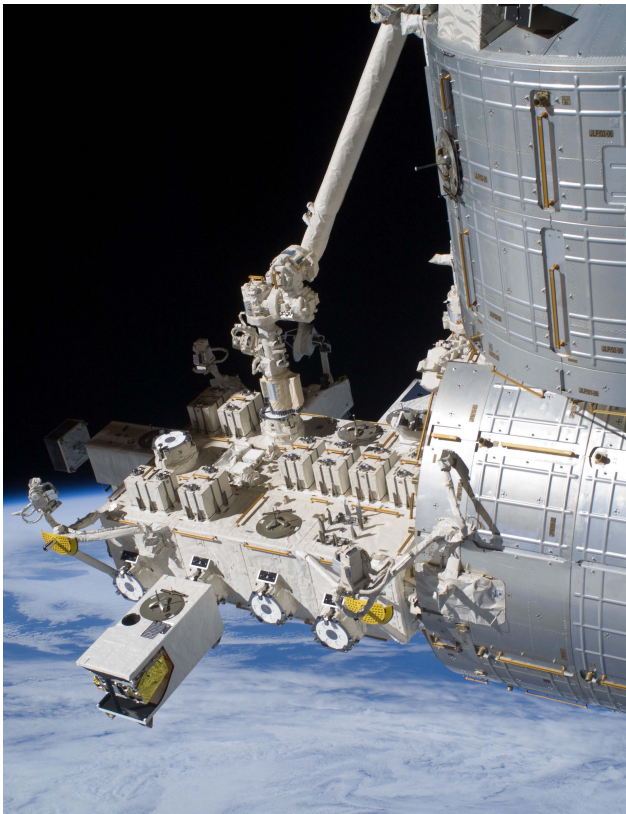
Figure 1. The Japanese Experiment Module-Exposed Facility (JEM-EF) on the International Space Station. Payloads, such as CATS, attach using "plug-in" ports located around the JEM-EF. Image credit: NASA
