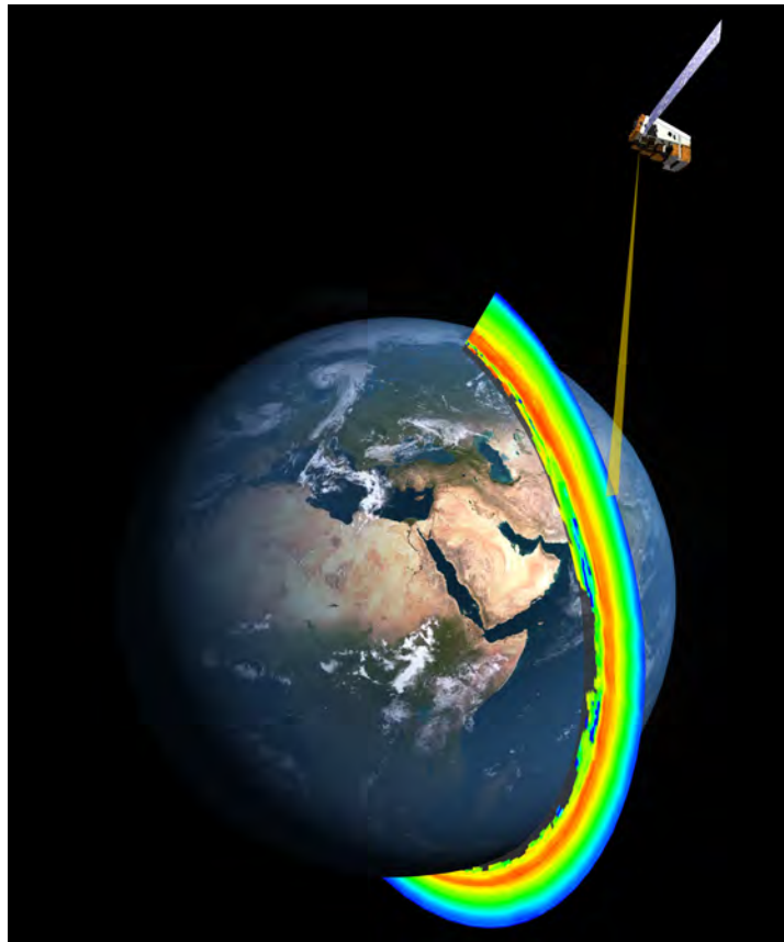
A cross-section of the Earth's ozone layer as measured by the limb profiler , part of the Ozone Mapping and Profiler Suite that's aboard the Suomi NPP satellite. A new instrument, the limb profiler makes high-vertical-resolution measurements of the ozone layer , a shield that protects the Earth's surface from the sun's dangerous ultraviolet radiation. Image credit: NASA/NOAA
