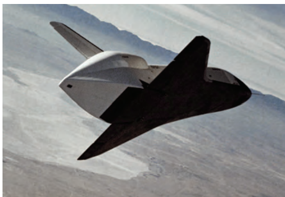
In this photo taken on September 26, 1977, during an aeronautical flight test, the Space Shuttle Enterprise is shown in free flight after separation from a Boeing 747 airliner modified for use as a shuttle carrier aircraft. Image Credit: NASA
