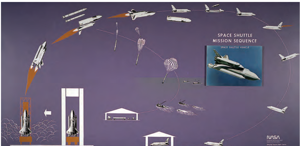
This diagram, from 1975, illustrates the space shuttle mission sequence. Image Credit: NASA
