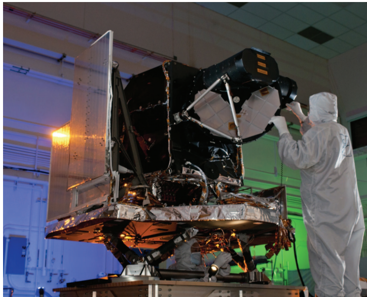
The Operational Land Imager (OLI) being integrated onto the LDCM spacecraft. Photo Credit: Ball Aerospace Technology Corporation
