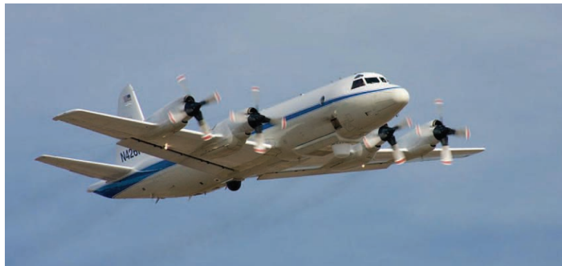
Figure 1. NASA's P-3B is a four-engine turboprop, capable of long-duration flights of 8–12 hours. It is based at NASA's Wallops Flight Facility. Image credit: NASA
