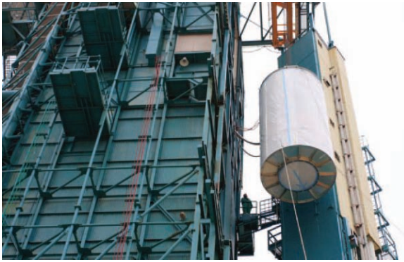
An overhead crane lifts the Aquarius/SAC-D spacecraft, secured inside its payload transportation canister, into the mobile service tower at NASA's Space Launch Complex-2 (SLC-2) at Vandenberg Air Force Base in California. Aquarius, the NASA-built instrument on the SAC-D spacecraft, will provide new insights into how variations in ocean surface salinity relate to fundamental climate processes on its three-year mission. Image credit: NASA VAFB
