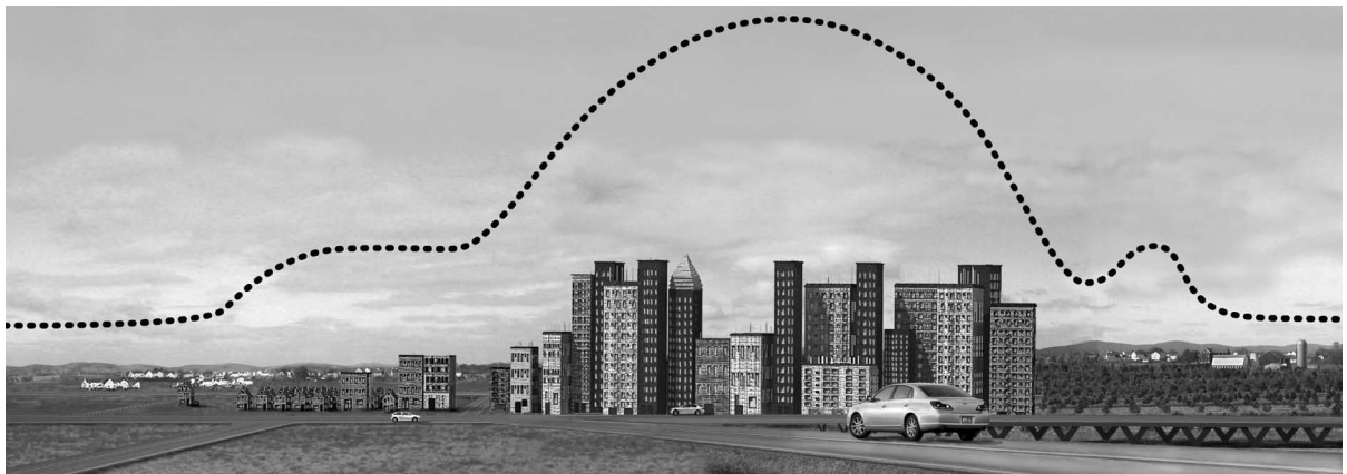
The urban heat island effect can raise temperatures within cities as much as 9°F (5°C) higher than the surrounding countryside. New data suggests that the effect is more or less pronounced depending on the type of landscape—i.e., forest or desert—the city replaced. Credit: NASA
