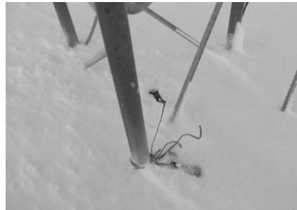
Three Thermocron ibuttons placed on the snow surface to monitor the surface temperature and compare to the 2-m air temperature.
