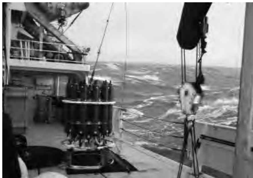
The CTD on the deck of the Ron Brown against a backdrop of whitecap covered ocean, a sight rarely seen at the study site.
