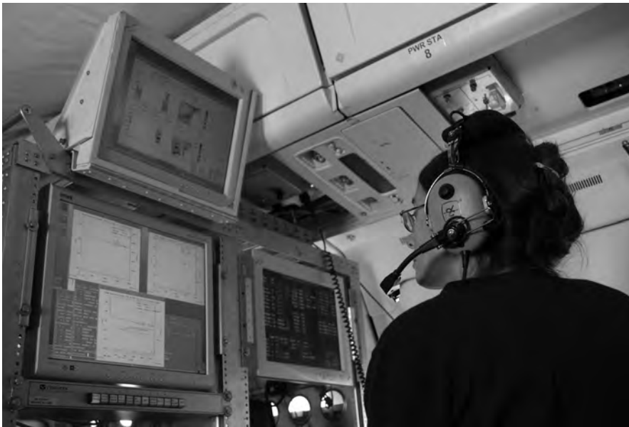
Susan Kool monitors data from the Lidar Atmospheric Sensing Experiment (LASE) instrument on board a NASA DC-8 aircraft flying through a Saharan dust storm over the Atlantic. Researchers hope to use these data to track interactions between the dust and tropical storms and to better understand Atlantic hurricane development. Photo courtesy: NAMMA team.
