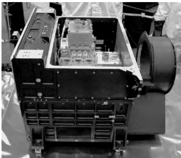
A photo of the Aerosol Polarimetry Sensor as it was being assembled at Raytheon.
