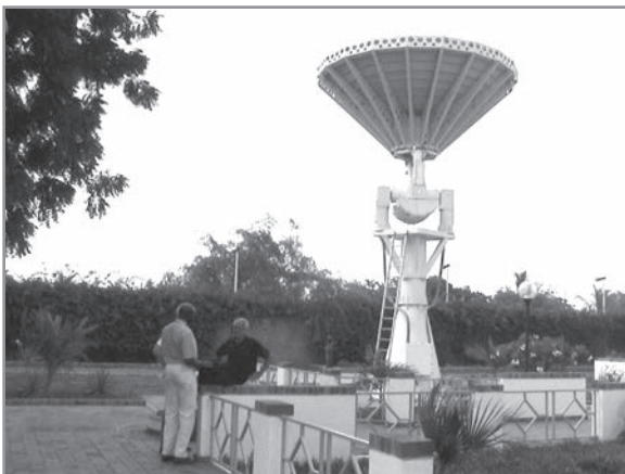
Figure 5. The 6.1 m X-band antenna of the Remote Sensing Centre, Broglia Space Center, Malindi. This dish can receive EOS Terra/MODIS and Aqua data in direct broadcast mode. Photo by Charles Gatebe.
