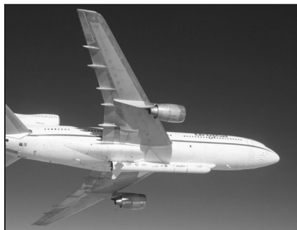
The L-1011 and the Pegasus climbing to 40,000 feet — the elevation required for the drop.
